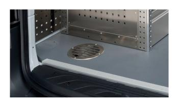
It is essential to take care when installing ventilation and venting grids on parts of the frame, electrical and/or hydraulic lines, fuel lines or fuel tanks, other floor openings etc.!
