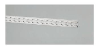
ALUCA fastens the lashing rails with M6 countersunk screws (DIN 7991) of strength 8.8 and M6 locknuts (DIN 985) or M6 expansion nuts. With a spacing of approx. 150 mm, we can guarantee pull-out force of 200 daN. We have demonstrated this by means of pull-out trials of the lashing rails in collaboration with the manufacturer.
