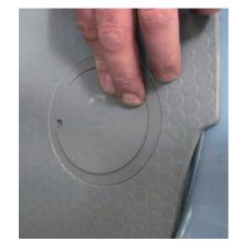
Refix the lashing point with original screws
