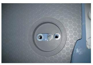
Set the hole with a stepped drill; compensate for unevenness with bodywork spacers (ø 20 mm) (not in the deliverables)
