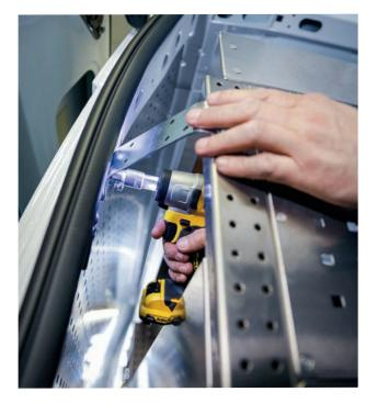
The wall fastenings must be fixed so that they are evenly loaded in tension and pressure. If the device has more than 2 supporting frames, the central fastening frame must also be fixed. Use M6 expanding rivet nuts with collar. In each case, two screws must always be fixed to the supporting frame and to the bodywork.
