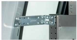
Please adhere precisely to the instructions for fixing the wall fastening brackets, as these are important for fastening the device securely in the vehicle! Tighten screwed connections with a torque according to the torque table (see p. 21). Mark screwed connections with a permanent marker according to the torque.
