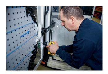
The side walls are delivered customised for your vehicle. We recommend that you stick felt strips to the rear of the side wall cladding or apply silicone, in order to avoid noises caused by vibrations occurring occasionally.
